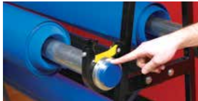
Safety collars and yellow security bars secure rollers and prevent injury
