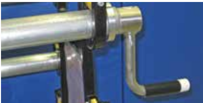
Two hand cranks with rotating grips for easy winding
